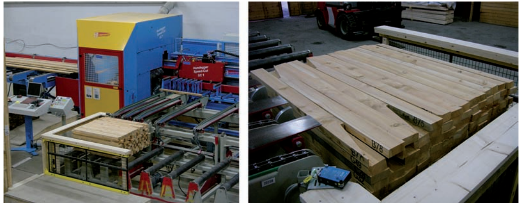
Figure 5 The Hundegger SpeedCut SC1 CNC machine used by Kjeldstad Sagbruk & Høvleri AS to produce the nearly 700 timber components for the Ringve Botanical Garden viewing platform. All components were automatically labeled with the machines ink lettering unit. Without this numbering system it would not have been possible to assemble the structure.
